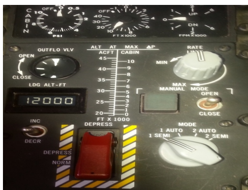
Fig 8. Pressurisation control panel
