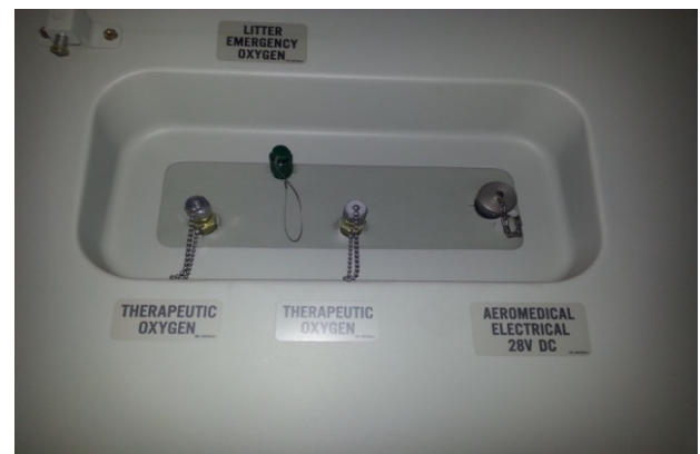
Fig 5. Oxygen outlets to supply aeromedical litter stations
