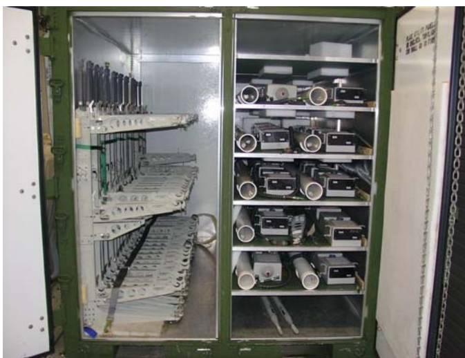
Fig 4. LSAS container to carry litters and utility panels
