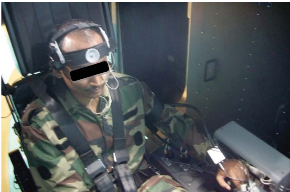
Fig-1: Subject sitting in HPHC cockpit with TCD probe secured on head
