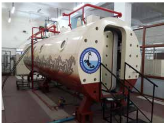
Fig 1. Rapid Recompression Chamber at IAM IAF
