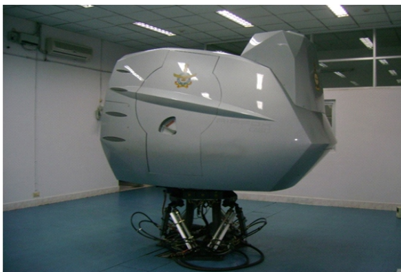
Fig-1: Airfox® Spatial Disorientation Simulator
