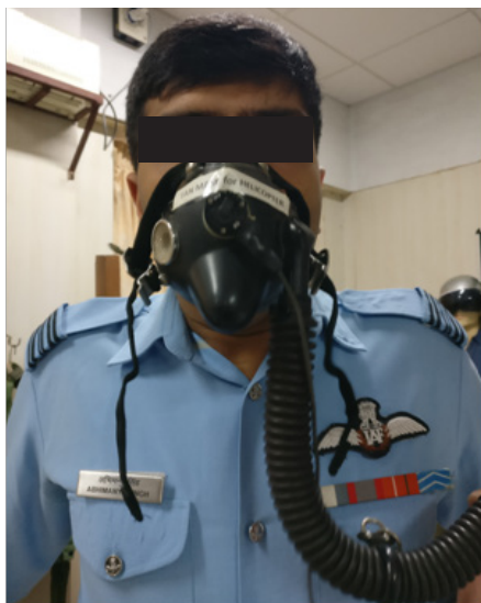
Fig 4. Ability to create a vacuum after the inlet hose was closed. Displays adequate seal between edge of mask & face.
