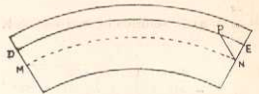
Fig. 4 Strain in a bent bar
