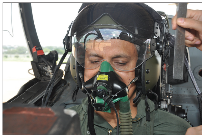
Figure 3: Cockpit trial depicting visor mask gap.
