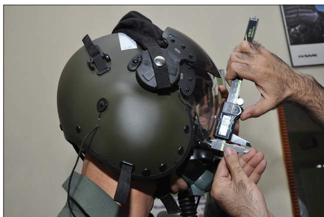
Figure 2: Measurement of gap between visor and mask with vernier caliper.
