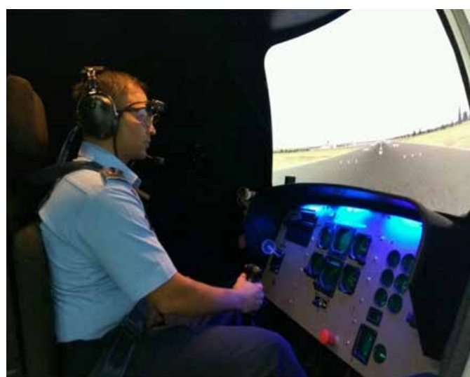
Fig 3. Eye scan patterns recording in Airfox DISO® SD simulator
