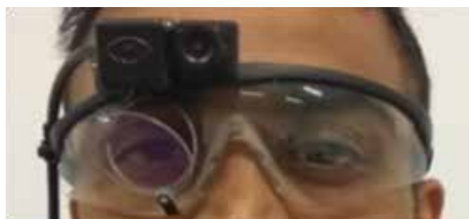
Fig 2. A subject wearing the ASL® mobile eye tracker
