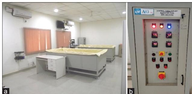
Figure 1: (a and b) Dry supine immersion tanks with control unit.
